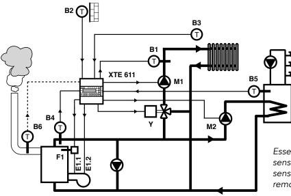
Essential sensors: 1 outside sensor, 1 heating flow sensor, 1 boiler sensor. Optional accessories: 1 room sensor, 1 DHW sensor, 1 or 2 flue gas sensors, 1 remote control.
